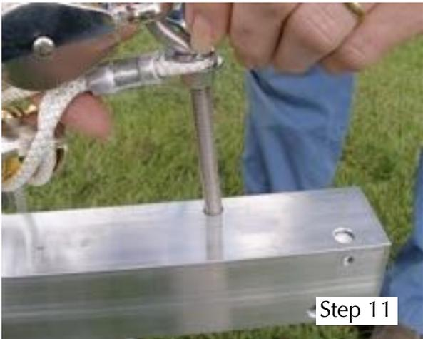
Thread the lock nut back on and tighten the nut all the way to the pole. Make sure that you orient the eyebolt so that open end is facing up, and that the eyebolt is parallel to the pole. See photo 11A. Push your hub
