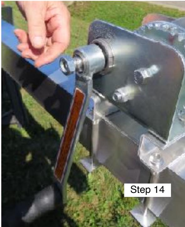
**Step 15)** From the mounting kit box get the Safety Pin (N) and remove the hitch pin (M) that is in place by grasping the large rounded loop and pull. Insert the hitch pin into the hole that is in your lower pole section (A) about 6 feet from the ground up. Replace the hitch pin and push the pin all the way thru so that the curved part of hitch pin, where you grasped it is in all the way.
