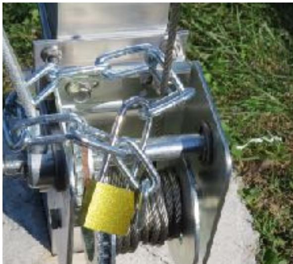
of chain (Q). Remove the packing from the lock, and in order to open the lock you will need to remove one of the keys on the key ring. Open the lock. Take the chain wrap it so that it goes around the winch handle behind the cable, and then with the hasp of the lock insert it through the chain links both ends. Close the lock.
