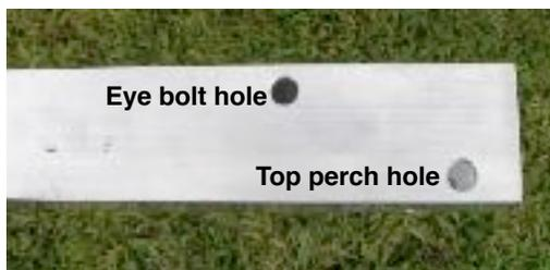
**Step 3** Basically you are taking the parts you removed and re-inserting them into their appropriate holes in the extension piece. Start by re inserting the top perch rods, re use your set screws and tighten. Place the black cap into the top of the pole. Lastly re insert the eyebolt into the pole.
