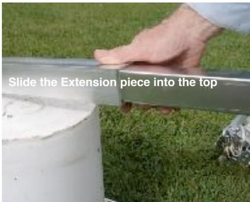
**Step 2.** Pole assembly: Once all the parts are removed from the top section of the 14 foot pole, slide the extension piece into the top of the pole and lay the pole on an overturned 5-gallon bucket (or similar object). The 3 pole pieces are held in place by friction and gravity.
