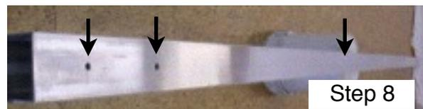
whiz nuts (V) Insert the bolt by inserting arm into the aluminum hub and push the bolt thru the hole in the center of the hub, one bolt for each of the 4 sides of the hub, and thread the whiz nut on so your bolt wont fall off. Do not tighten the nuts.
