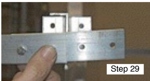
ets. Thread on the nut. Repeat the process on the other side of the ring section you just attached. DO NOT tighten the bolts just yet.
