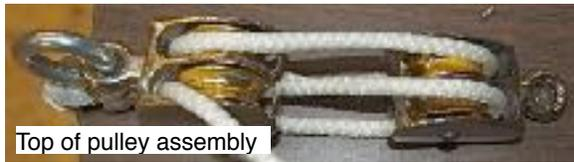
pulleys eye onto your quick link as seen in the photo. Close the quick link and tighten using a 1/2 inch open end wrench. Remove the lock nut from the end of the eyebolt and place the threaded end of the eyebolt into the eyebolt hole on the pole. Replace the lock nut back on to the end of the eyebolt, and tighten the lock nut to the pole using a 9/16" wrench. Your rope should look EXACTLY like the photo 14B.
