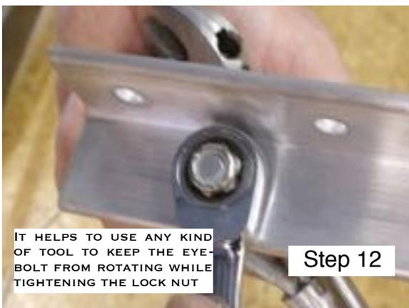
IT HELPS TO USE ANY KIND OF TOOL TO KEEP THE EYE-BOLT FROM ROTATING WHILE TIGHTENING THE LOCK NUT
