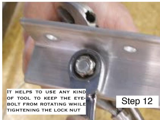
**Step 12)** Arm/eyebolt attachment. Find your arm that has the eyebolt hole (E) in it and your cable that has the eyebolt attached to it (K). Remove the lock nut from the end of the eyebolt. Insert eyebolt into the hole, thread lock nut back on till it meets the angle, and tighten using your 9/16" socket wrench. Orient the eyebolt so that it is parallel to the arm.
