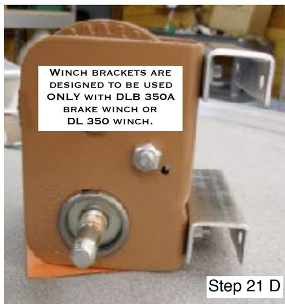
WINCH BRACKETS ARE DESIGNED TO BE USED ONLY WITH DLB 350A BRAKE WINCH OR DL 350 WINCH.
