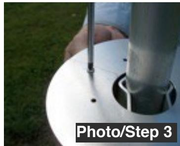
Step 3) Insert the other #8 x 3/8" screw and attach nut. Tighten both of these screws.
